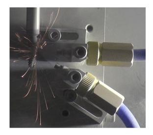
The ST200 system is an innovative solution for medical screws and dental implants texturing using abrasive media blasting.
